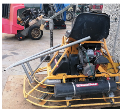
Dynapac concrete helicopter
